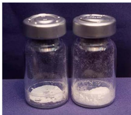
Collapsed Product – Critical Temperature Was Exceeded
