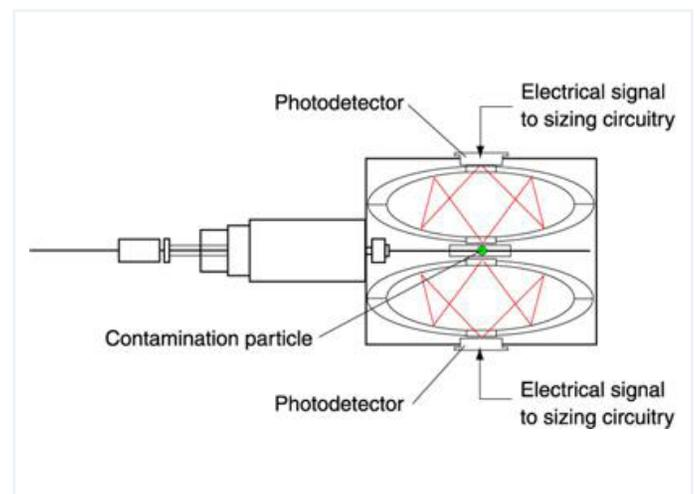
**Figure 4:** Light Scattering Particle Counter - Principle Credit: PMT (GB)
